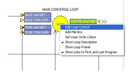
Note that the typical application of the NJRTM-E would not require any modifications to the main convergence loop control. The model will terminate automatically if the convergence criteria are achieved or if the model processes the maximum number of iterations permitted by the user.
