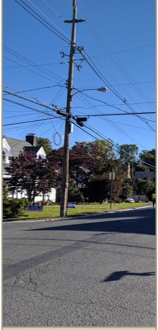
Figure 21. Overhead cobra lighting, as pictured, is found along the study corridor.
