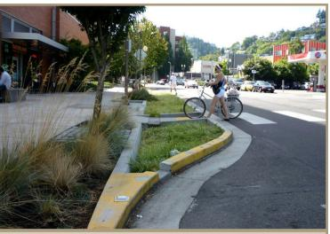
*Figure 10. Green infrastructure used to narrow the roadway and provide a shorter crossing distance for pedestrians.*
