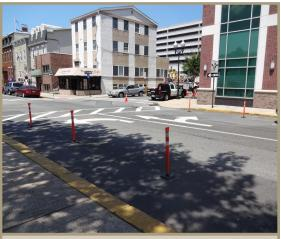
*Figure 46. New Brunswick, NJ, uses plastic bollards to prevent illegal parking near intersections.*
