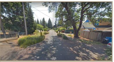
*Figure 43. Green infrastructure used to narrow the roadway in Philadelphia, PA.*
