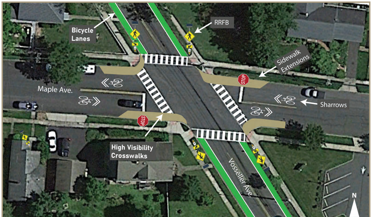
Figure 40. Proposed recommendations, including bicycle lanes, shared lane markings, curb extensions, high-visibility crosswalks, and RRFBs.
