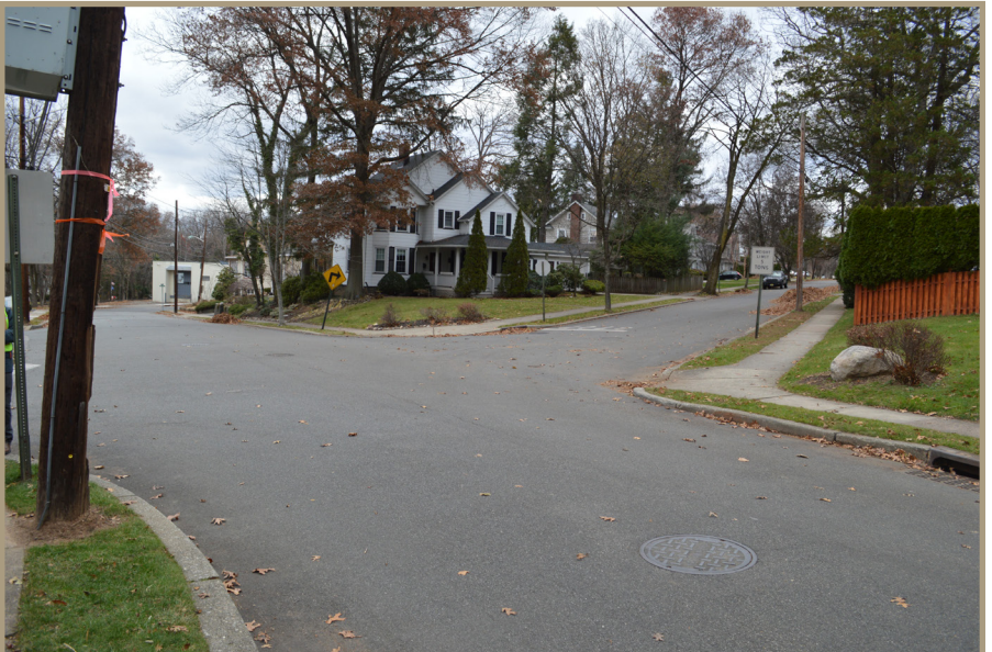
Figure 26. Crosswalks are not painted in any direction (looking northeast).
