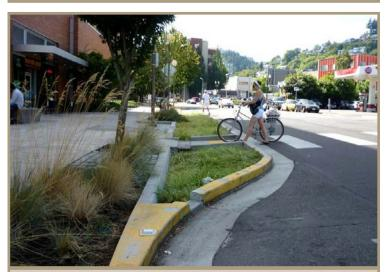
Figure 9. Green infrastructure used to narrow the roadway and provide a shorter crossing distance for pedestrians.
