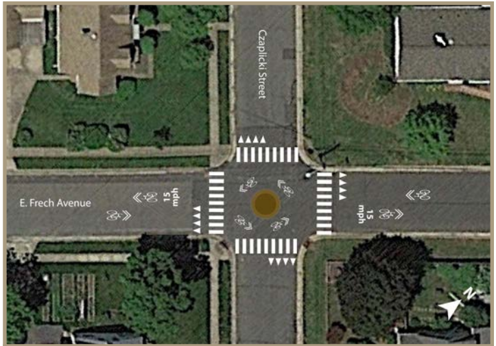
Figure 40. The intersection of E. Frech Avenue and Czaplicki Street with proposed Bicycle Boulevard improvements.
