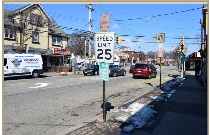
Figure 22. Cluttered sidewalks with hazardously low signage, looking northward on North Beverwyck Road near the intersection of Hiawatha Boulevard.
