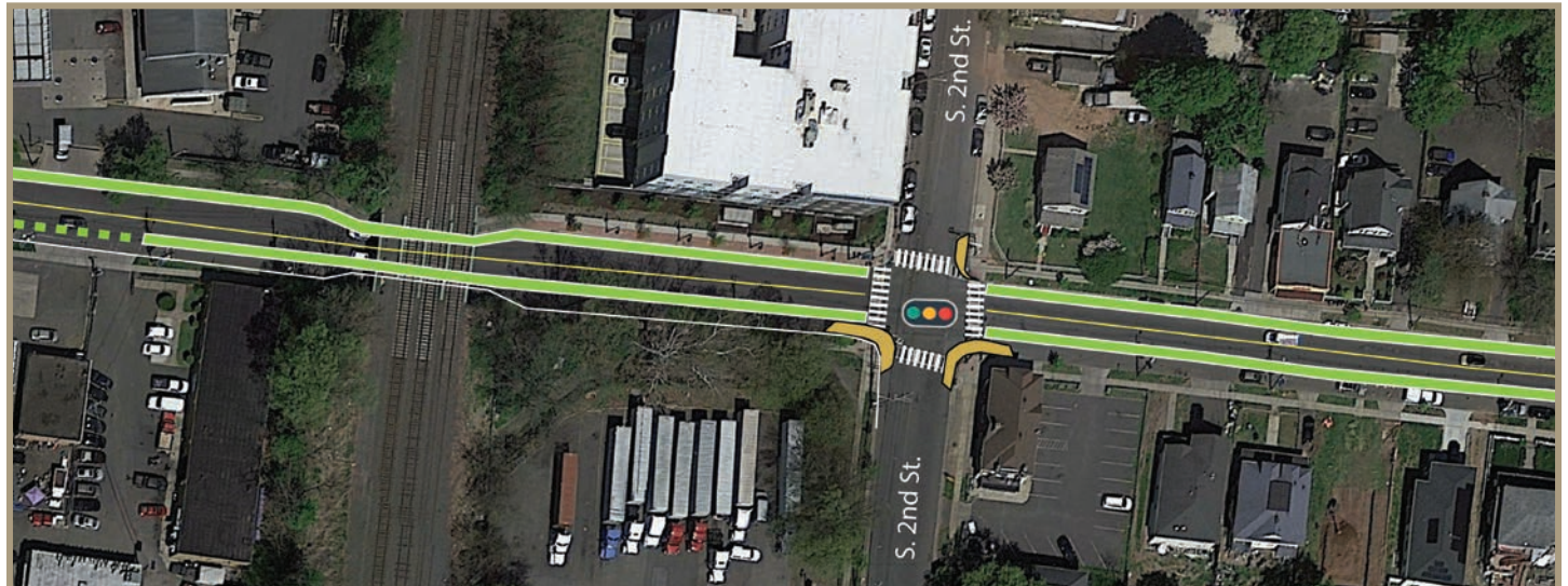
Figure 15. Plan showing proposed bicycle lanes, marked crosswalks and curb extensions added to Grant Avenue.
