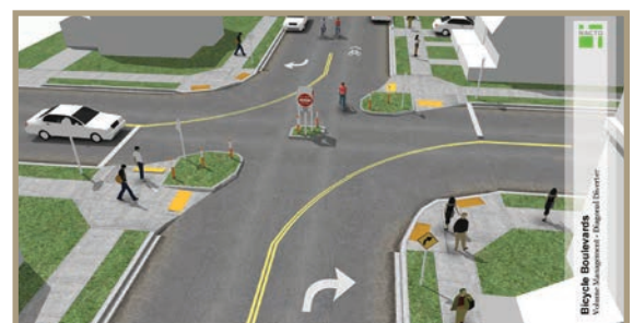
Figure 25. A diagram of a traffic diverter with pass-through for bicycles and pedestrians. Source: NACTO.
