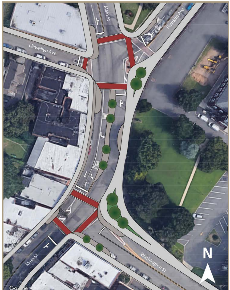
Figure 77. Alternative 2: Reconfiguring the intersections.
