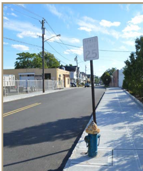
Figure 20. Brand new sidewalk on Columbia Street is wide and even, but lacks trees.
