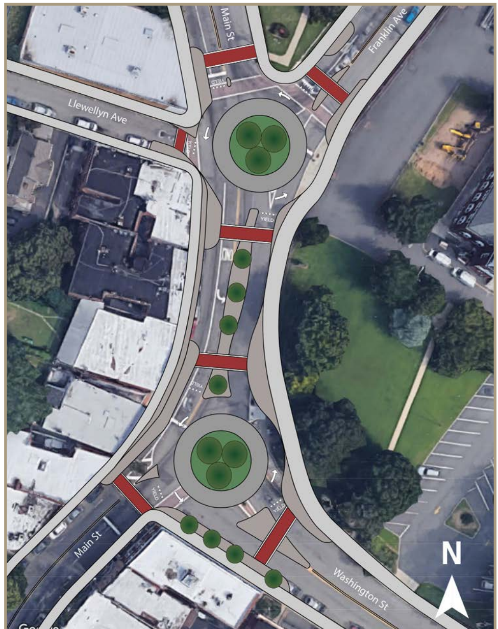
Figure 78. Alternative 3: Two modern roundabouts
