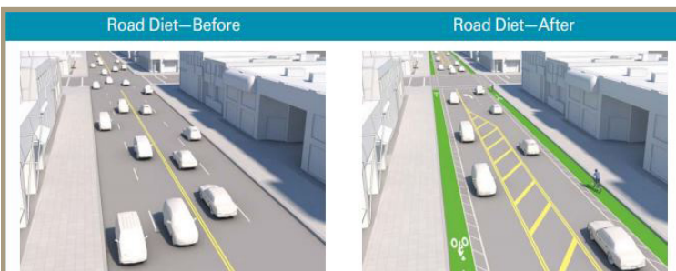
Figure 49. Road diet before and after as depicted in the New Jersey Complete Streets Design Guide.
