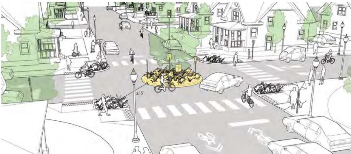
Figure 13 – Single Lane Mini-Roundabout in Neighborhood Example (Source: NATCO)
