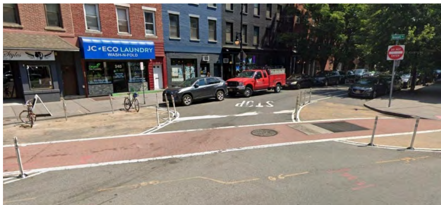
Figure 10 – Painted Curb Extension Example, Jersey City (Source: Google)
