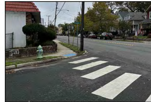
Building and vegetation obscures sight distance
