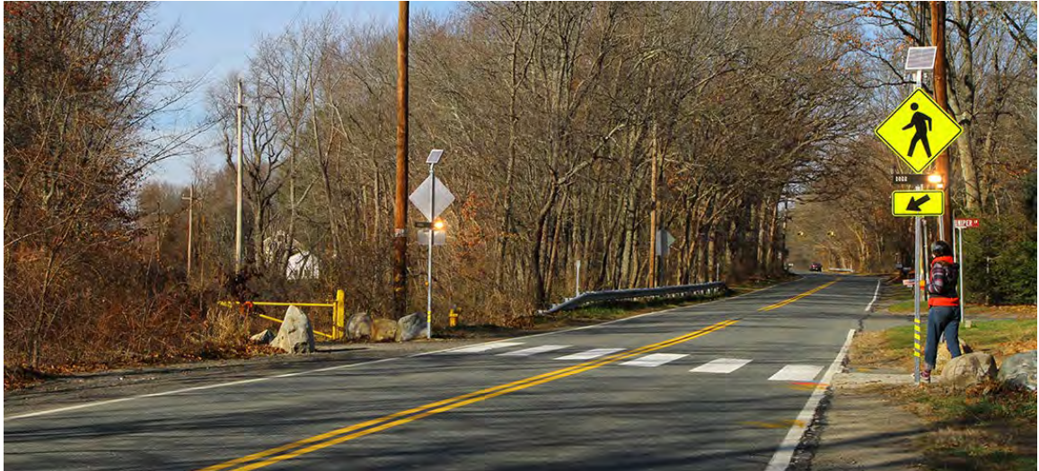
Figure 7 – RRFB at Trail Crossing (Source: Carmanah)
