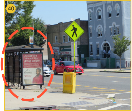
Sight distance for Parkhurst Street eastbound is limited by bus shelter
