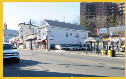
The gas station at the Madison Avenue intersection has three driveway entrances, one of which is very close to the intersection. There are several crashes that involved vehicles utilizing this driveway.
