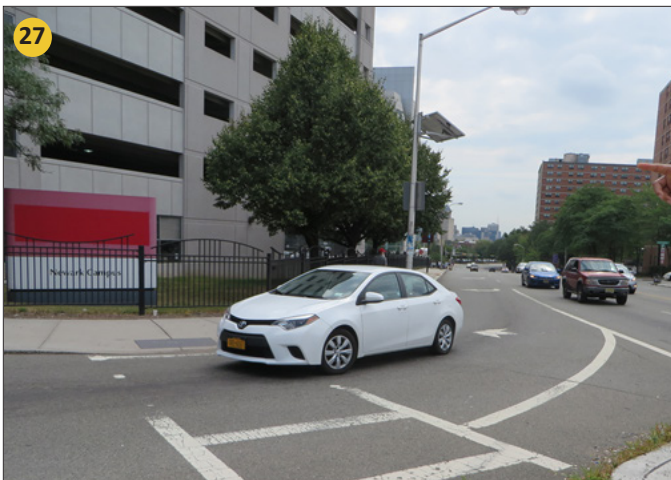
Wide slip ramp allows vehicles to access Bergen Street at high speeds. Motorists were observed not yielding to pedestrians. There is no advance warning sign of pedestrians on the slip ramp, and the sight triangle on approach is limited by fencing.
