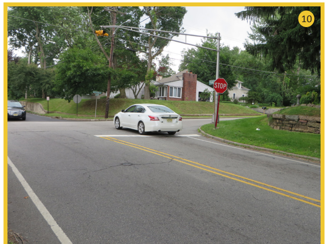
Figure 46 – Encroaching vehicles due to poor sight triangle
