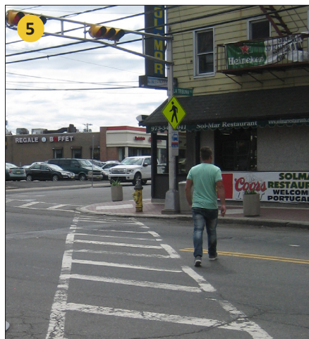
Antiquated signal equipment; lack of pedestrian signal heads
