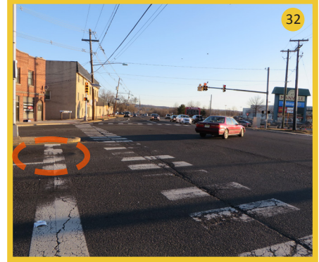
The median island on west leg is an obstacle for turning radius
