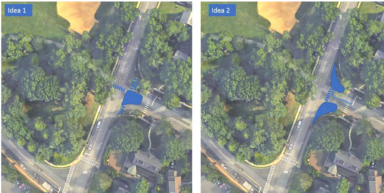
Figure 12 – Recommendation at South Crescent. Left: Crossing Island. Right: Curb Extension.
