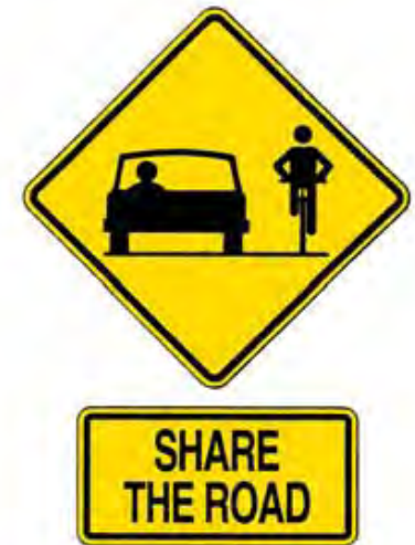
Shared Lane Signage
