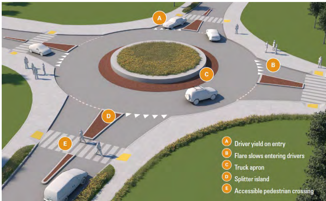
Figure 21 – Roundabout Example (Source: CSDG)
