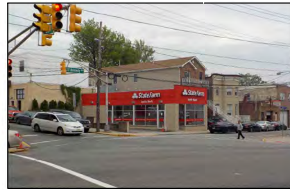
Crosswalks do not align with pedestrian signal heads and locations block visibility of / for pedestrians (Similar intersection has different marked crosswalk locations)
