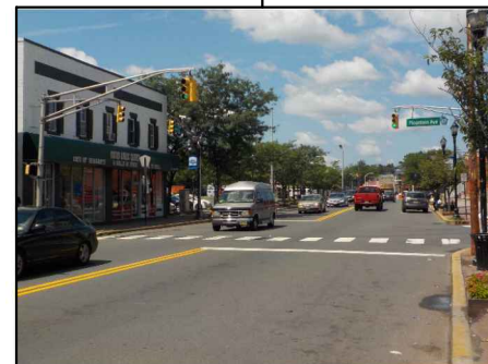
8-inch signal heads difficult to see
