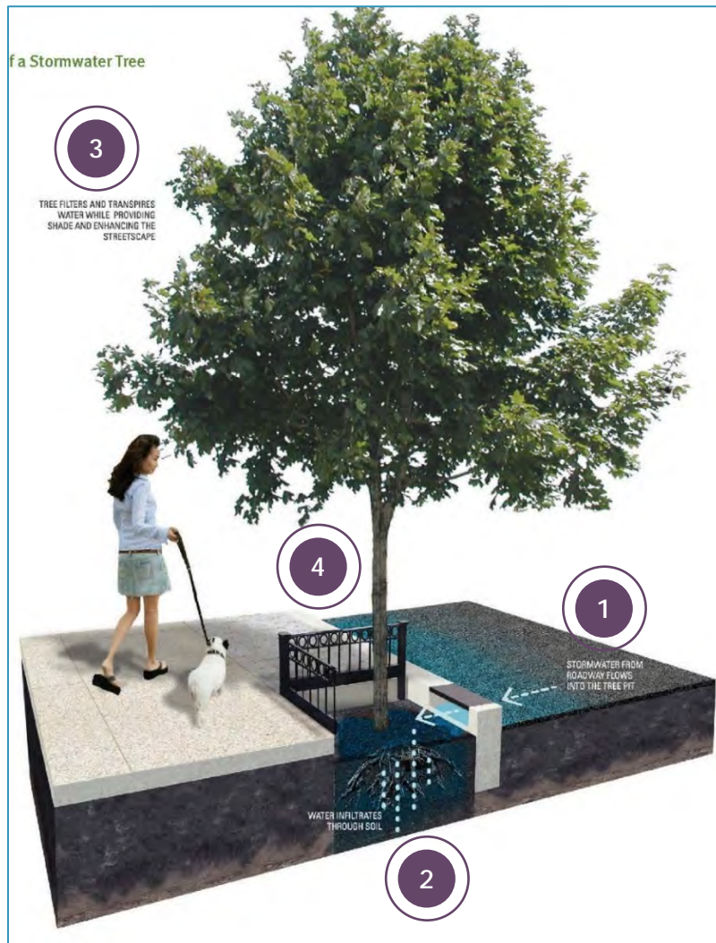
Figure 14 – Stormwater Tree Well Example (Source: City of Philadelphia Green Streets Design Manual)
