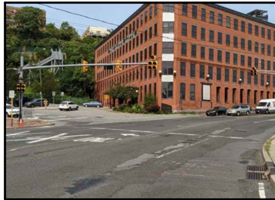
Optically programmed signalheads may not be aligned to oncoming traffic
