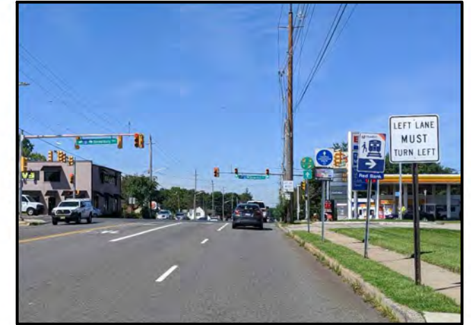
Multiple signs in succession may not be interpreted by drivers in time to make decisions
