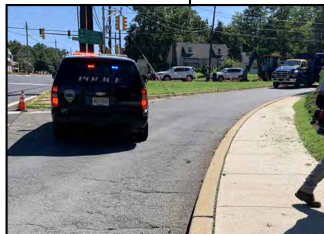
Channelized right turn lacks place for pedestrians to cross
