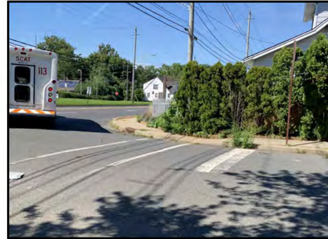
Bushes may block sight distance for side street turning vehicles
