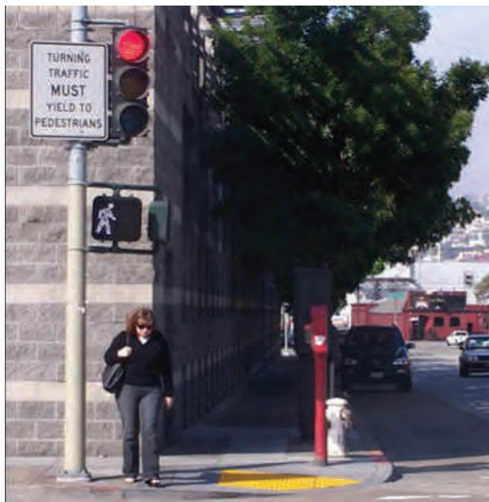
A leading pedestrian interval allows pedestrians to begin crossing the intersection before vehicles, improving pedestrian visibility and increases crossing time. Source: fhwa.gov
