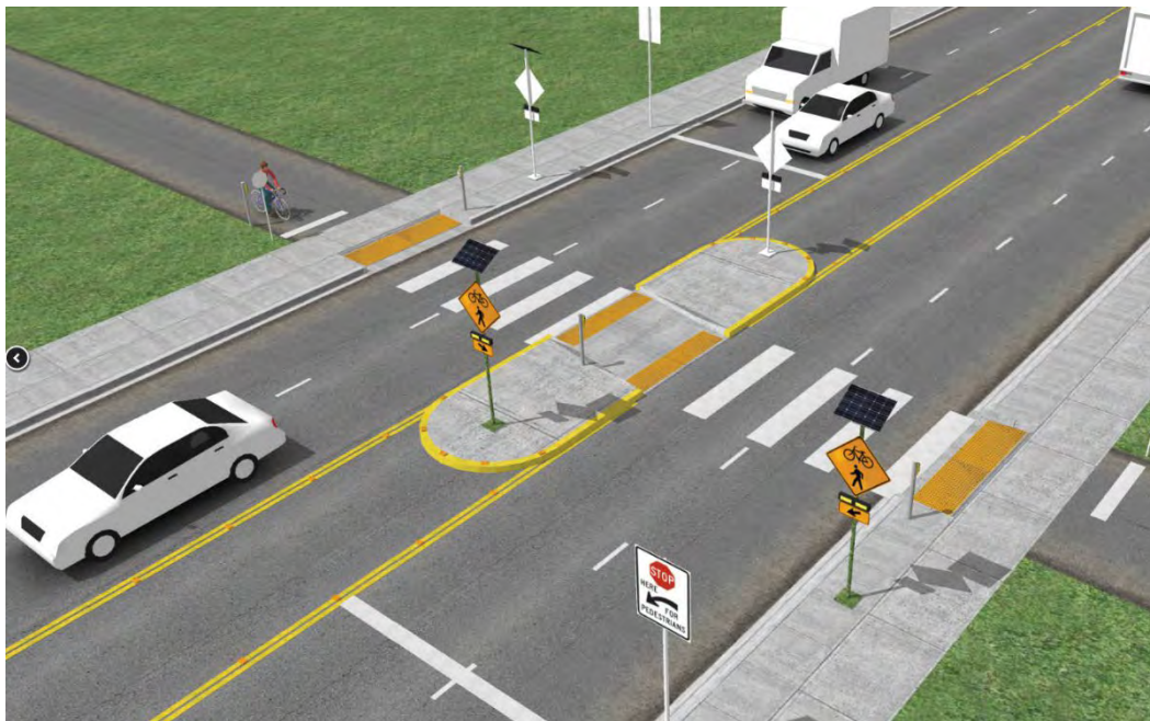
Figure 13 - Example of a Rectangular Rapid Flashing Beacon (Source: NACTO-Urban Bikeway Design Guide)
