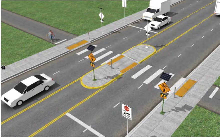
Figure 12 - Example of a Rectangular Rapid Flashing Beacon (Source: NATCO: UB)
