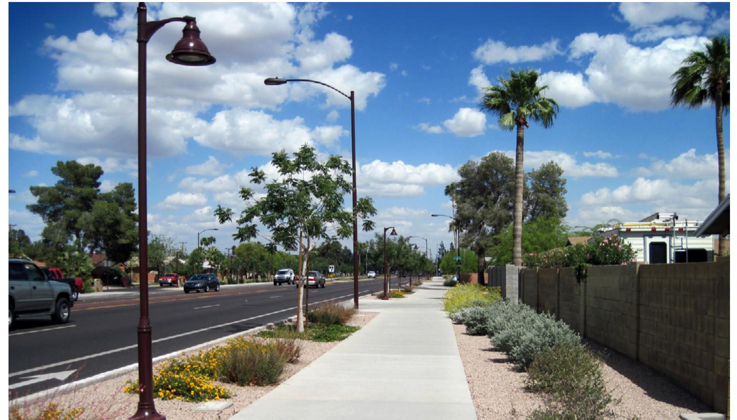
Figure 23: Pedestrian-scale lighting faces the sidewalk in this example in Scottsdale, Arizona (Image Source: Achen Gardner & City of Scottsdale, AZ)
