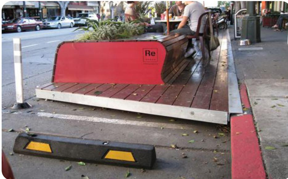
Safety components like wheel stops and the reflective bollard are used to protect this San Francisco, CA parklet<sup>56</sup>
