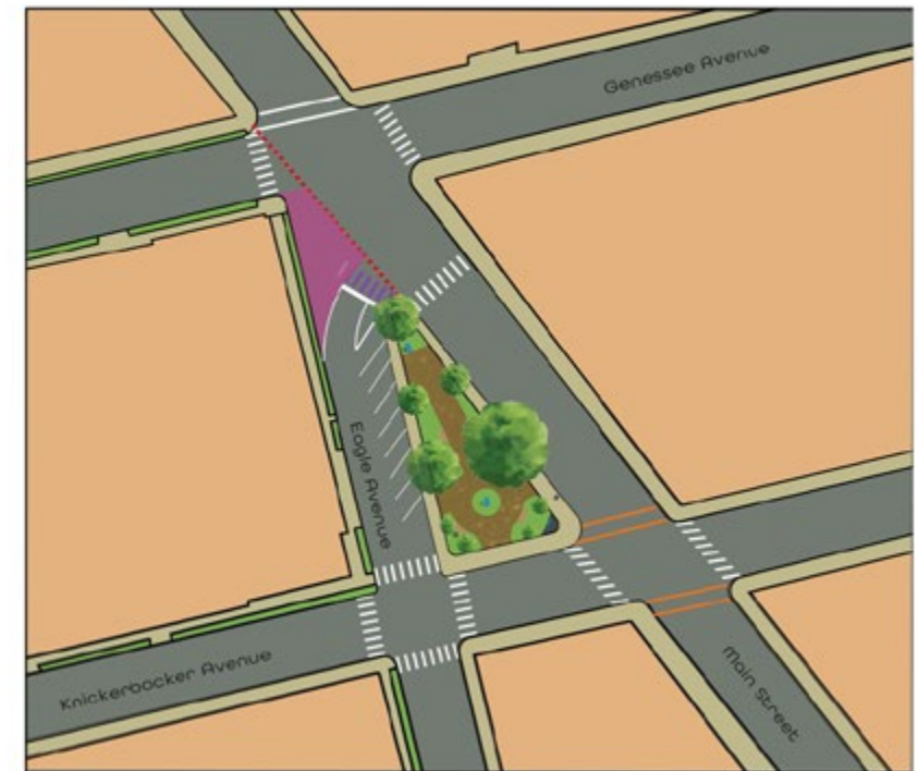
FIGURE 25 OPTION FOR RECONFIGURATION OF CROSSING ON THE NORTH END OF MAIN & GOULD PARK.
