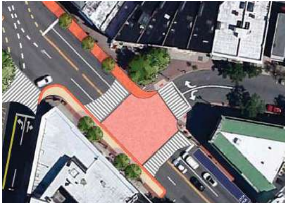
Intersection concept in Montclair Center - Intersection recommendations include curb bumpouts, ergonomic crosswalks, textured intersections & dedicated bus loading
