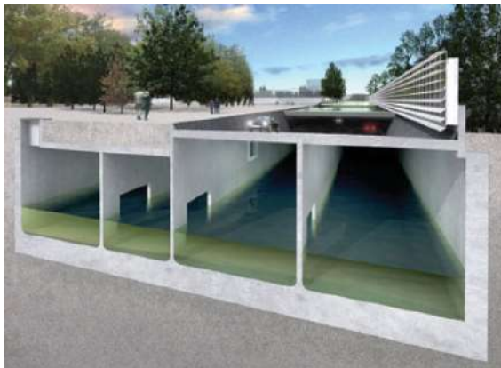
Rotterdam Museum park: Underground parking and stormwater storage
