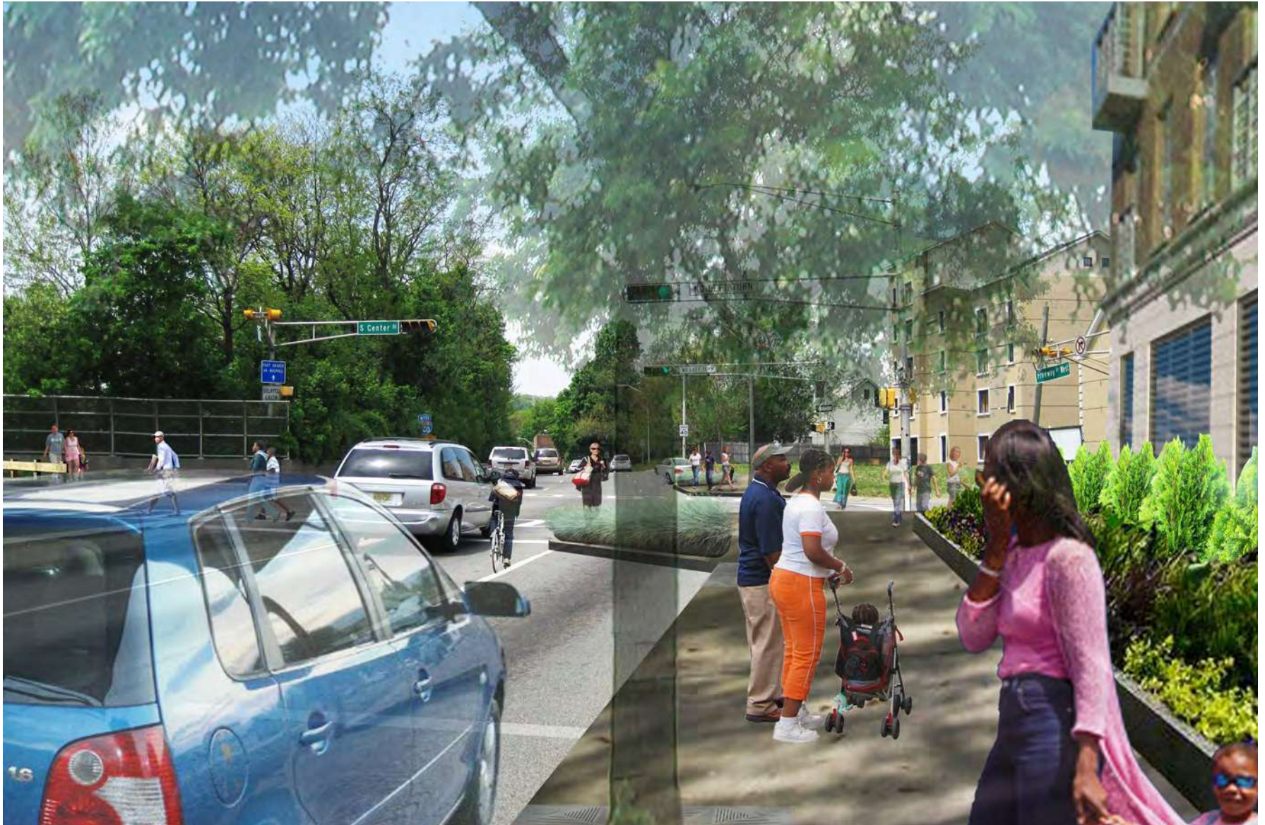
AFTER: This view at Center Street and Freeway Drive West shows how a few simple measures, such as converting one through-traffic lane to parallel parking, bulb-outs at the intersection, and street trees, could have a transformational effect in making Freeway Drive less of a pedestrian barrier, and, in improving the environment along Freeway Drive, can also help to attract development to the adjacent properties.
