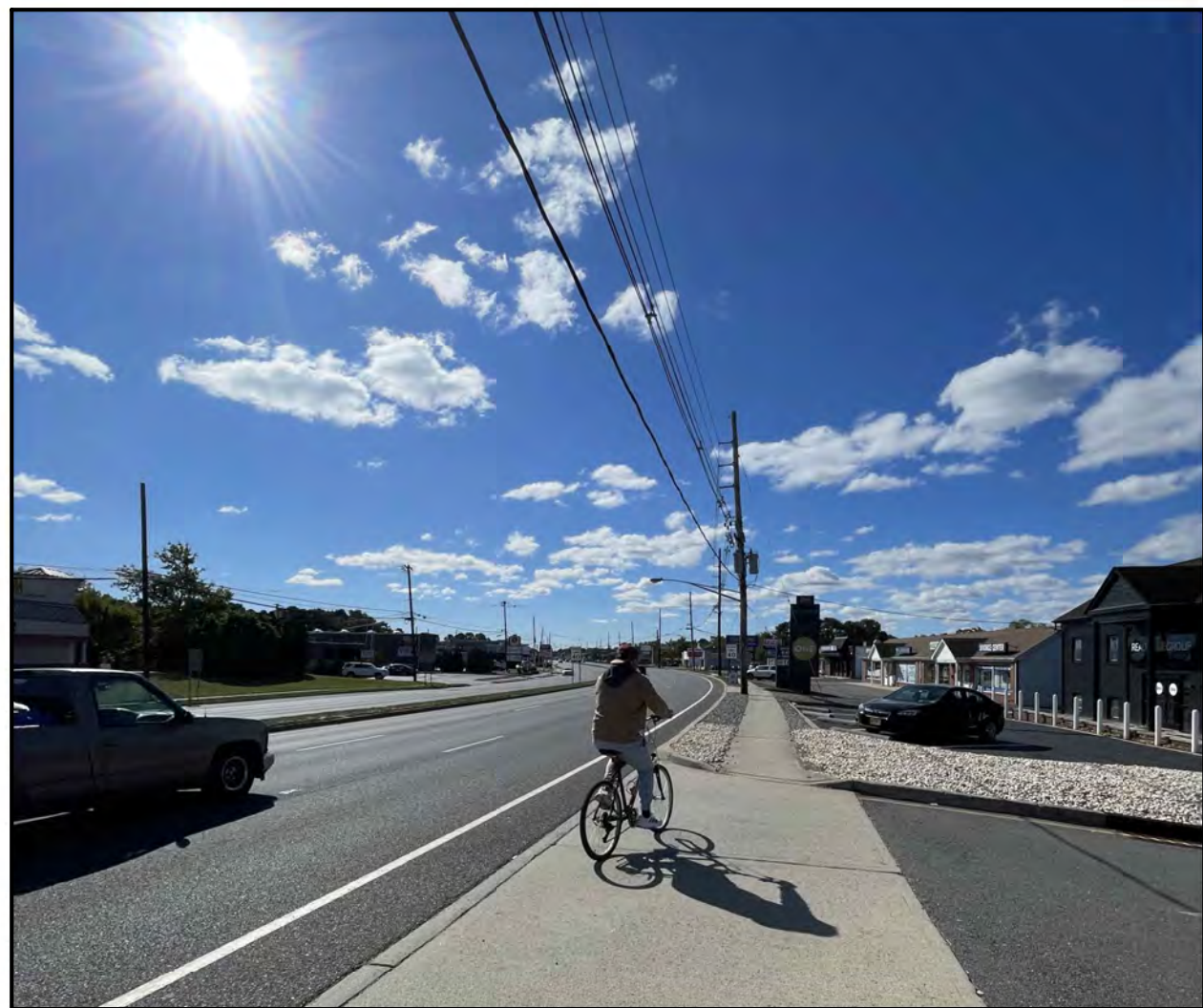
No bike lanes and small shoulder width forces bicyclist to use the sidewalk
