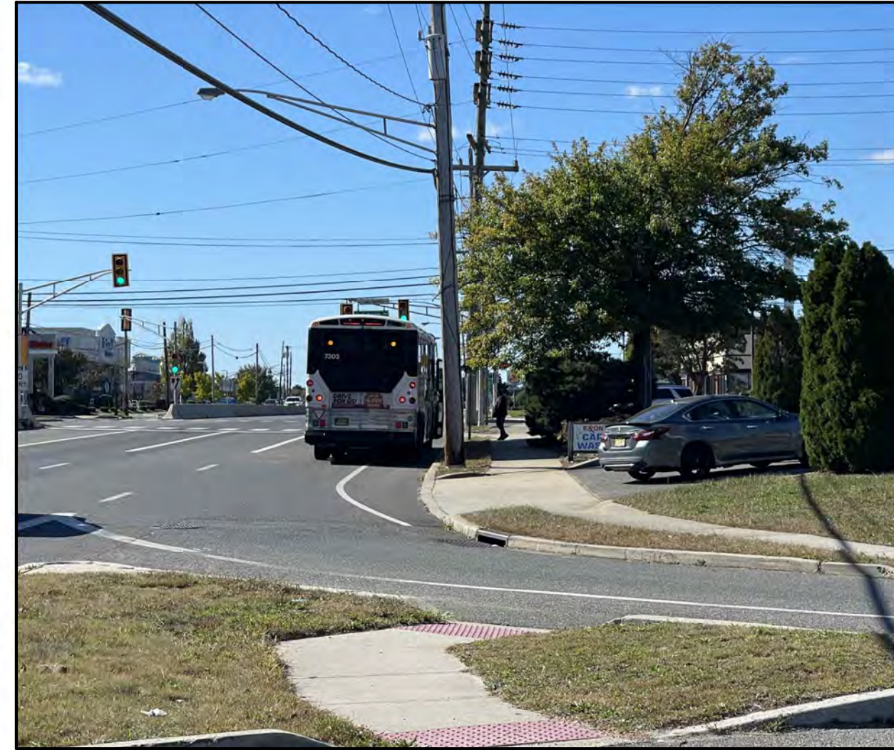
Bus stops are located at the intersection and obstructs the right lane when stopped
