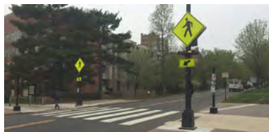
RRFBs and high visibility crosswalks, Princeton Township, Mercer County
