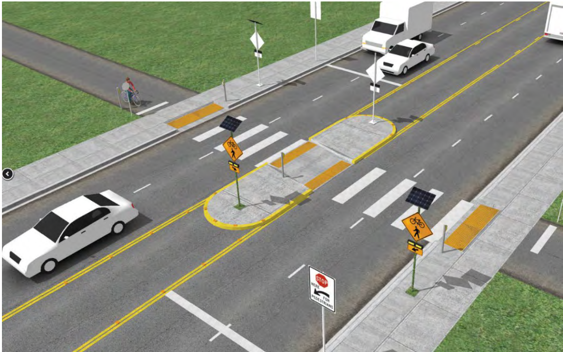
Figure 12 – Example of a Rectangular Rapid Flashing Beacon
